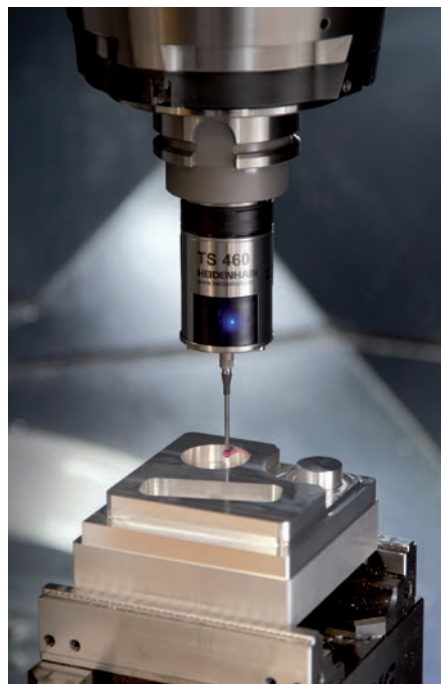
Measuring a circular pocket/hole
